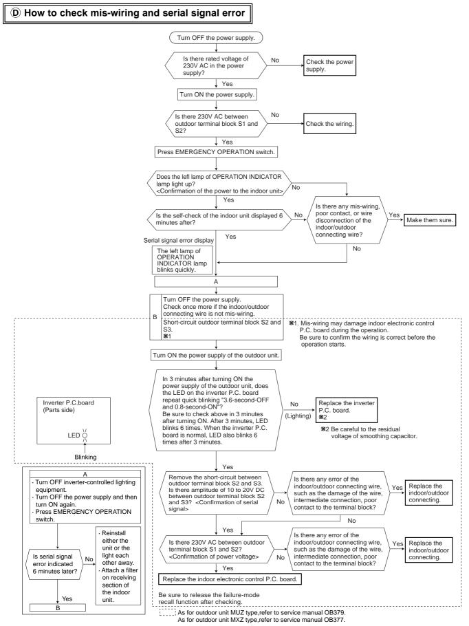
When All lamps flash ON and OFF every 0.5-second. Indoor unit and outdoor unit do not operate.
